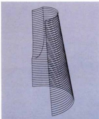
*The graphic representation of an air inlet duct was designed on the computer-based Numerical Geometry System.*
