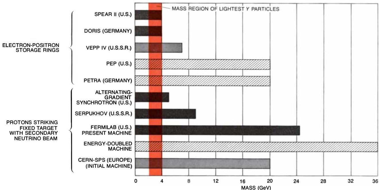
TEN PARTICLE ACCELERATORS capable of exploring the mass region of the  $Y$  particles will be operating in the next decade. Five of them are in operation now (black); two more are under construction (gray); the remaining three are being planned (hatched bars). In electron-positron storage rings particles collide with equal and opposite velocity; in the remaining accelerators neutrinos collide with nucleons in a fixed target. The masses given represent not
