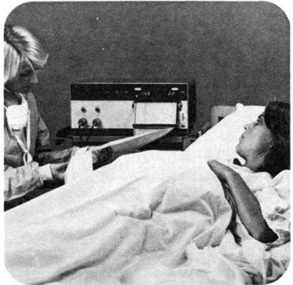
clearly identify the type of measurement method in use. An acceptance lamp lights with every valid heart rate measurement, and an INOP indicator immediately signals if there is any problem in the ECG electrode or transducer.
