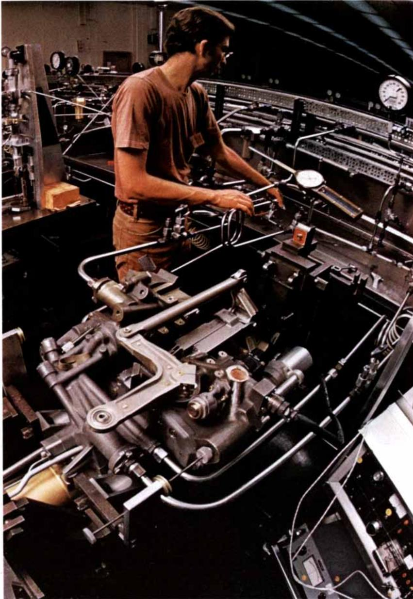
*At Berteia Corporation, an inboard elevator actuator package, designed with computer help, undergoes performance tests.*
