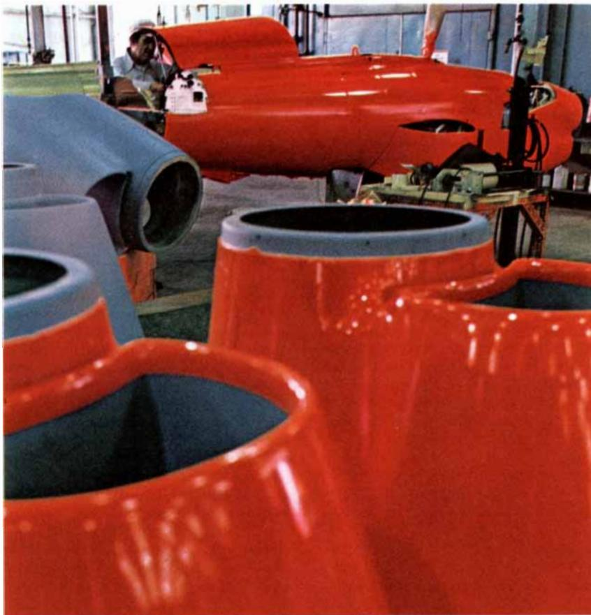
*The inlet duct graphically represented (below, left) is used in the Model 274 subsonic drone aircraft produced at Teledyne Ryan.*
