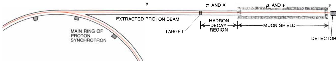
**BEAMS OF NEUTRINOS** are generated indirectly from protons accelerated in the 400-GeV proton synchrotron at the Fermi National Accelerator Laboratory (Fermilab). The protons collide with a metal target, generating pions and kaons. These mesons
