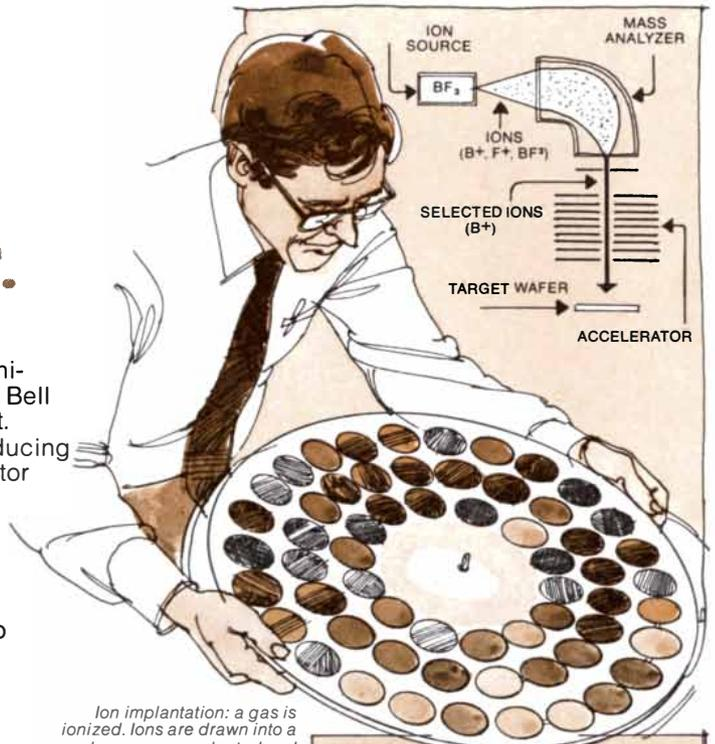
*Ion implantation: a gas is ionized. Ions are drawn into a beam, mass selected and implanted into target wafers.*
