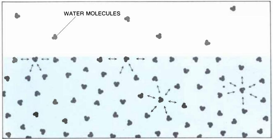
**SURFACE TENSION** of a liquid arises as a result of the unbalanced attractive forces that exist between molecules at the surface of the liquid. These forces, indicated here by two-headed arrows, are particularly strong between polar molecules, such as those of water, which have an asymmetrical distribution of electric charge. In the absence of gravity and air pressure the surface of a liquid will act as an elastic membrane, tending to minimize surface energy per unit area.
