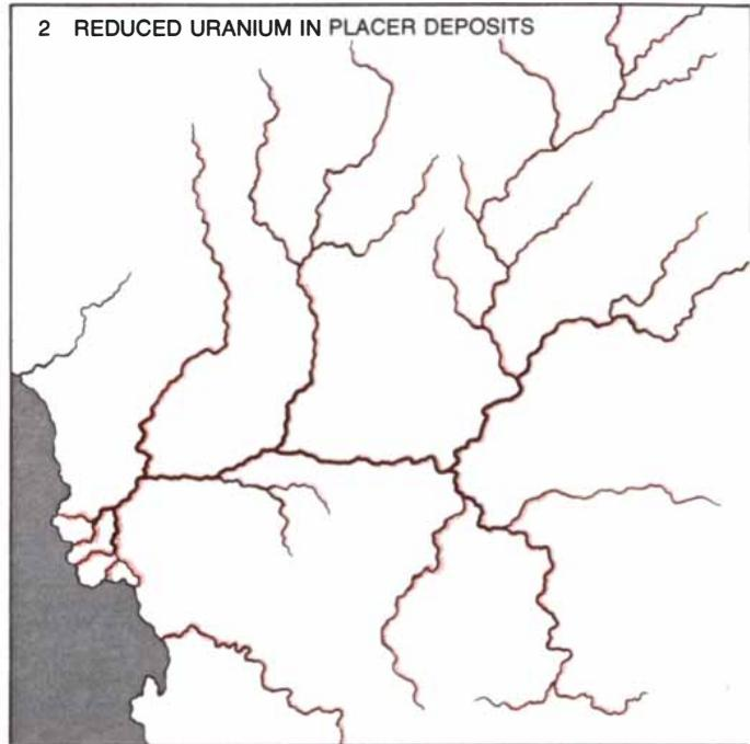
**ACCRETION OF THE ORE DEPOSIT** at Oklo involved the concentration of uranium derived from an entire watershed. The uranium (color) was originally dispersed in igneous rocks over a large area (1). As the rocks were eroded by weathering, the uranium accumulated in streambeds in a
