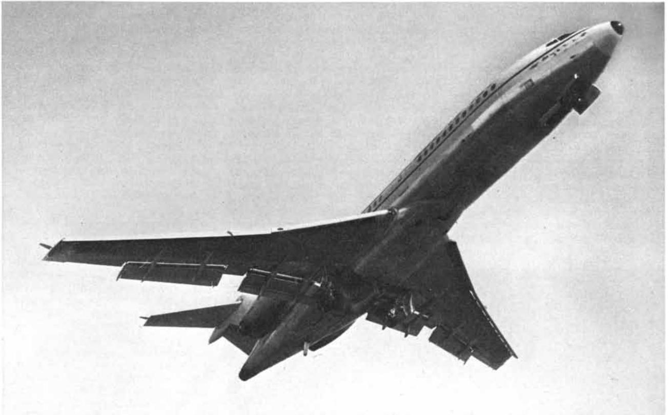
A Boeing 727 shortly after takeoff, with its triple-slotted trailing-edge flaps extended, from *Handling the Big Jets*
