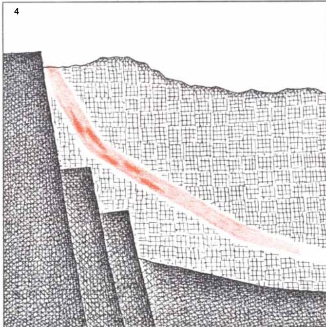
uranium had accumulated. For most of its history the ore was probably buried deep under other sedimentary rock, where it was protected from dissolution and dispersal by groundwater. Only much later, in the past few million years, did it approach the surface where it could be detected (4).
