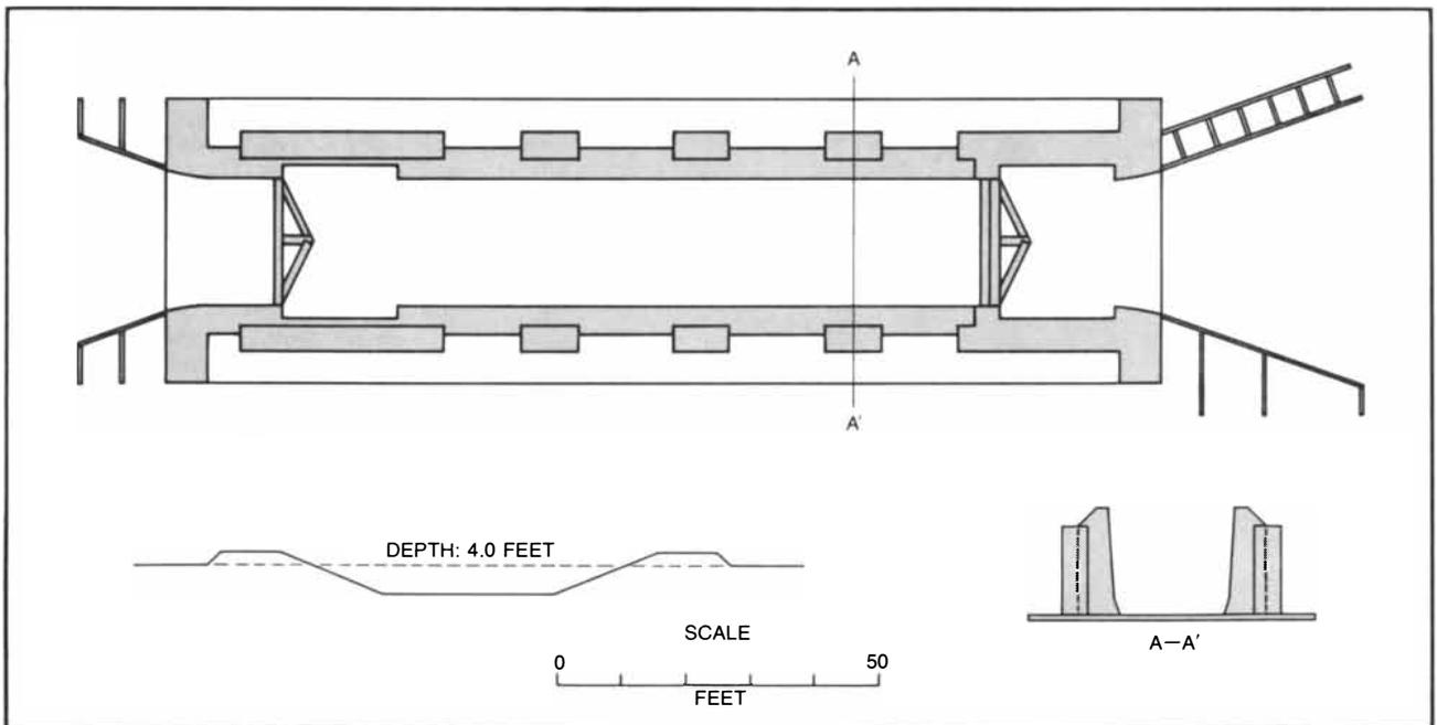
**LOCK ON THE ERIE CANAL** (top) and profile of the canal bed (bottom) are shown to the same scale in these simplified drawings based on contemporary plans. The V formed by the paired gates at each end of the lock points upstream; water pressure keeps the gates
