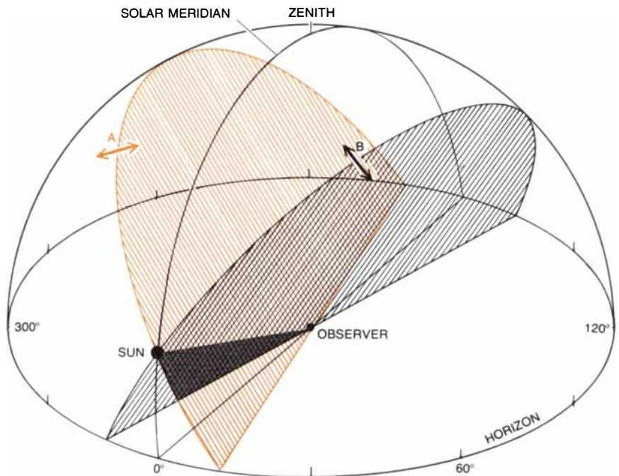
**AXIS OF POLARIZATION** (short two-headed arrows) of the light of the sky is always perpendicular to the plane of a triangle connecting the observer (center), the sun and the point in the sky being observed. The examples shown are for the points A and B on the celestial hemisphere. The planes of the great circles passing through the sun and each of the two points are hatched. Also shown is the solar meridian: the great circle passing through sun and the zenith.
