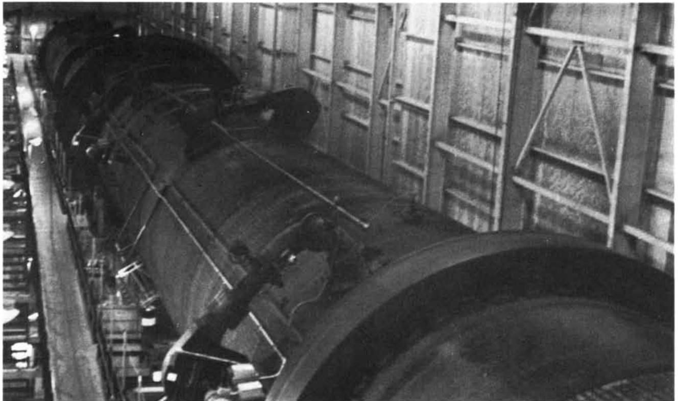
**ROTARY KILN** for the direct reduction of iron ore with a solid reductant is operated by the Steel Company of Canada, Ltd., in association with its own mine. Oxide pellets made from the iron ore magnetite serve
