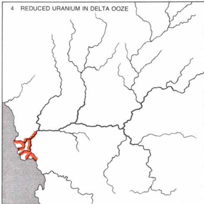
until it reached the delta of the river system, where sediments rich in organic ooze again created a condition of oxygen deficiency. In these sediments the uranium was returned to the reduced form and was precipitated out of the solution (4). In the delta the ore was covered by later sediments.
