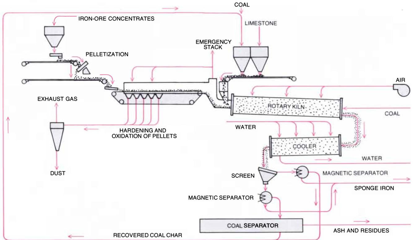
**SOLID REDUCTANT** is the distinguishing feature of the SL/RN direct-reduction process, which derives its name from the first letter of the name of each of four companies that helped to develop it. The reductant is coal, which consists mainly of carbon that reacts with the oxides in the iron ore. A mixture of ore, coal and limestone is fed into
