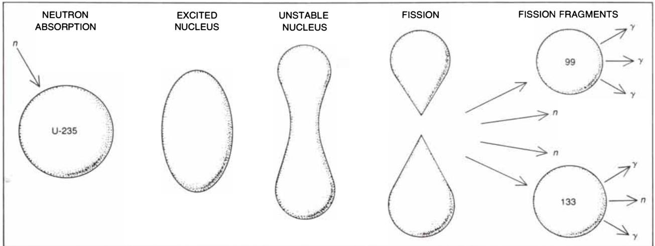
**FISSION OF A NUCLEUS** of U-235 is induced by the absorption of a thermal, or slow, neutron ( $n$ ), which excites the nucleus and deforms it. About 85 percent of the time the deformed nucleus becomes unstable and splits into two fragments of unequal size. The fission fragments shown have atomic mass numbers of 99 and 133; many other pairs of fragments are possible and each has a well-defined probabili-
