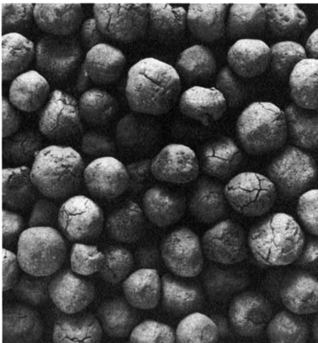
**IRON PELLETS** manufactured by the Midrex direct-reduction process at Sidbec plant are from two to three centimeters in diameter.
