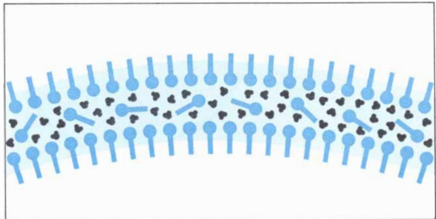
**SECOND IMPORTANT EFFECT** of soap on the formation of a liquid film is to limit the thickness of a film made from soapy solution to the length of two soap molecules stacked end to end.
