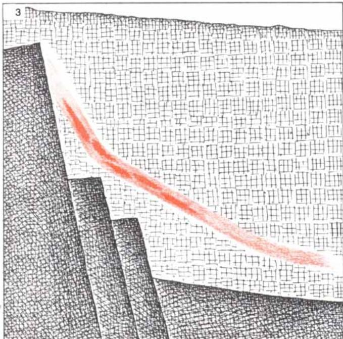
was tilted to its present average slope of about 45 degrees. The tilting caused numerous fractures, so that water could percolate through the ore, creating small pockets of very concentrated ore (3). In these pockets the chain reaction began as soon as enough
