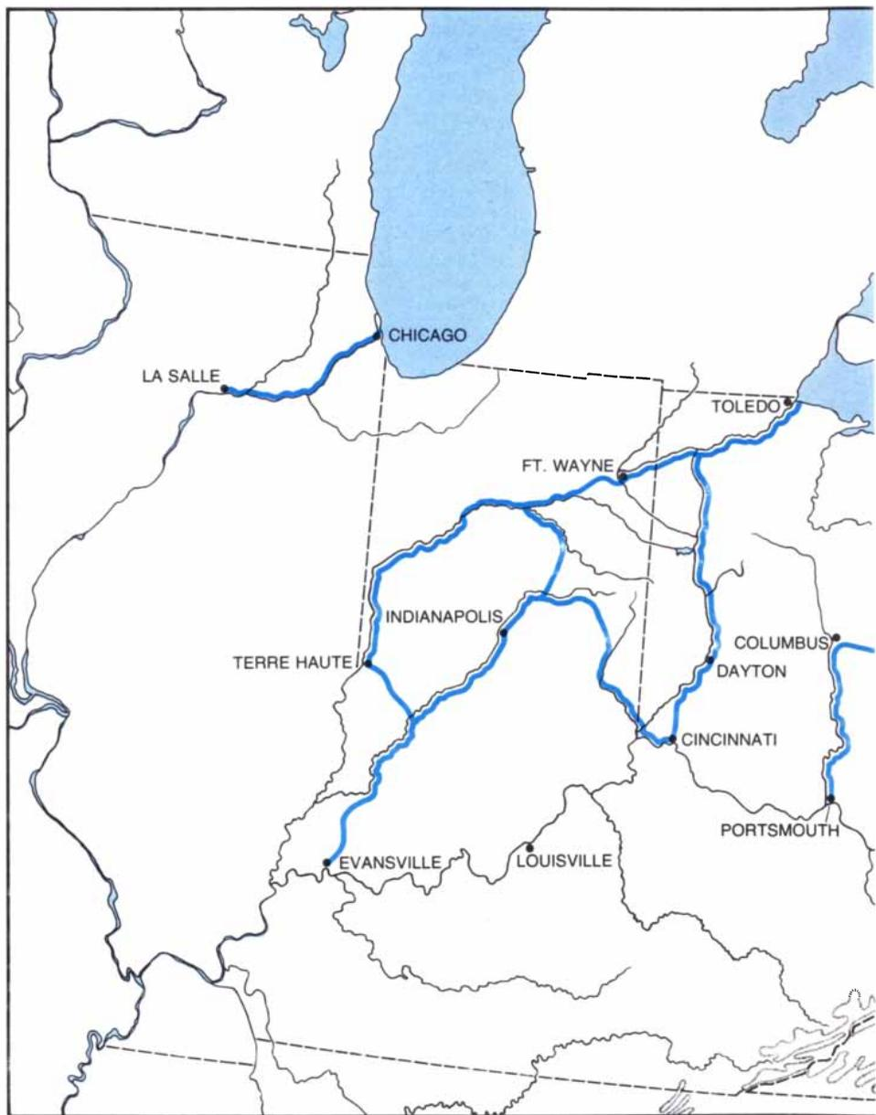
**NETWORK OF CANALS** constructed in the U.S., mainly between 1818 and 1860, was designed to attain two principal objectives. The earlier objective was to shorten or eliminate the coastwise movement of freight; an example is delivery of Pennsylvania coal via the Delaware and Hudson Canal and the Hudson River to New York, eliminating a voyage around New Jer-
