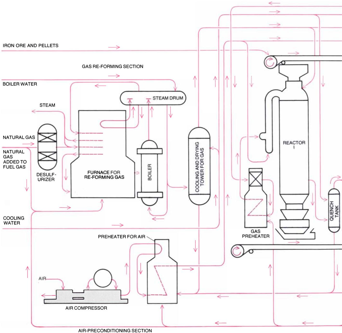
**HOJALATA Y LAMINA PROCESS**, usually abbreviated HyL, is named for the Mexican steel company that built the first plant incorporating the process in 1957. The process uses a gas to reduce iron ore, that is, to remove the oxygen that is associated with the iron in the ore, leaving the iron as a highly metallized material that can be made into
