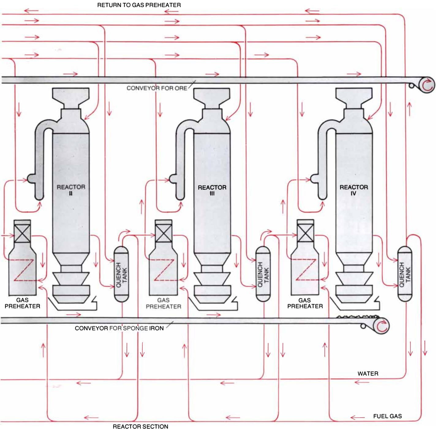
lets is loaded into the reactor from the top. During initial reduction preheated and partially spent gas from the reactor that has just completed final reduction is passed through the stationary bed of ore, preheating it and partly reducing it. In final reduction fresh, preheated gas from the reactor that is in the cooling stage is introduced, and the
