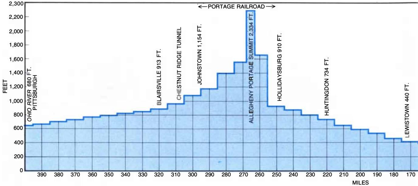
**PENNSYLVANIA CANAL PROFILE** shows a 2,334-foot lift from sea level at Philadelphia to the summit of the inclined-rail system connecting Hollidaysburg and Johnstown. The distance from Philadelphia to Pittsburgh was 400 miles; the first 90 miles of the system,
