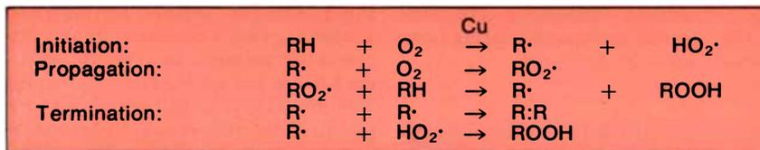
He pointed out that the rate of reaction of propagation and ultimate chain-length of cross-linking depend on the number of times the propagation step is repeated, i.e. the incidences of free radical promoters and amounts of available oxidants, which would include peroxides.
