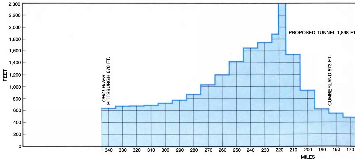
**CHESAPEAKE AND OHIO PROFILE**, as proposed, shows a lift from water level at Washington to 1,898 feet, where a four-mile tunnel was to be bored through the Allegheny Mountains some 215 miles west of Georgetown. Ground for the canal and for the Baltimore and
