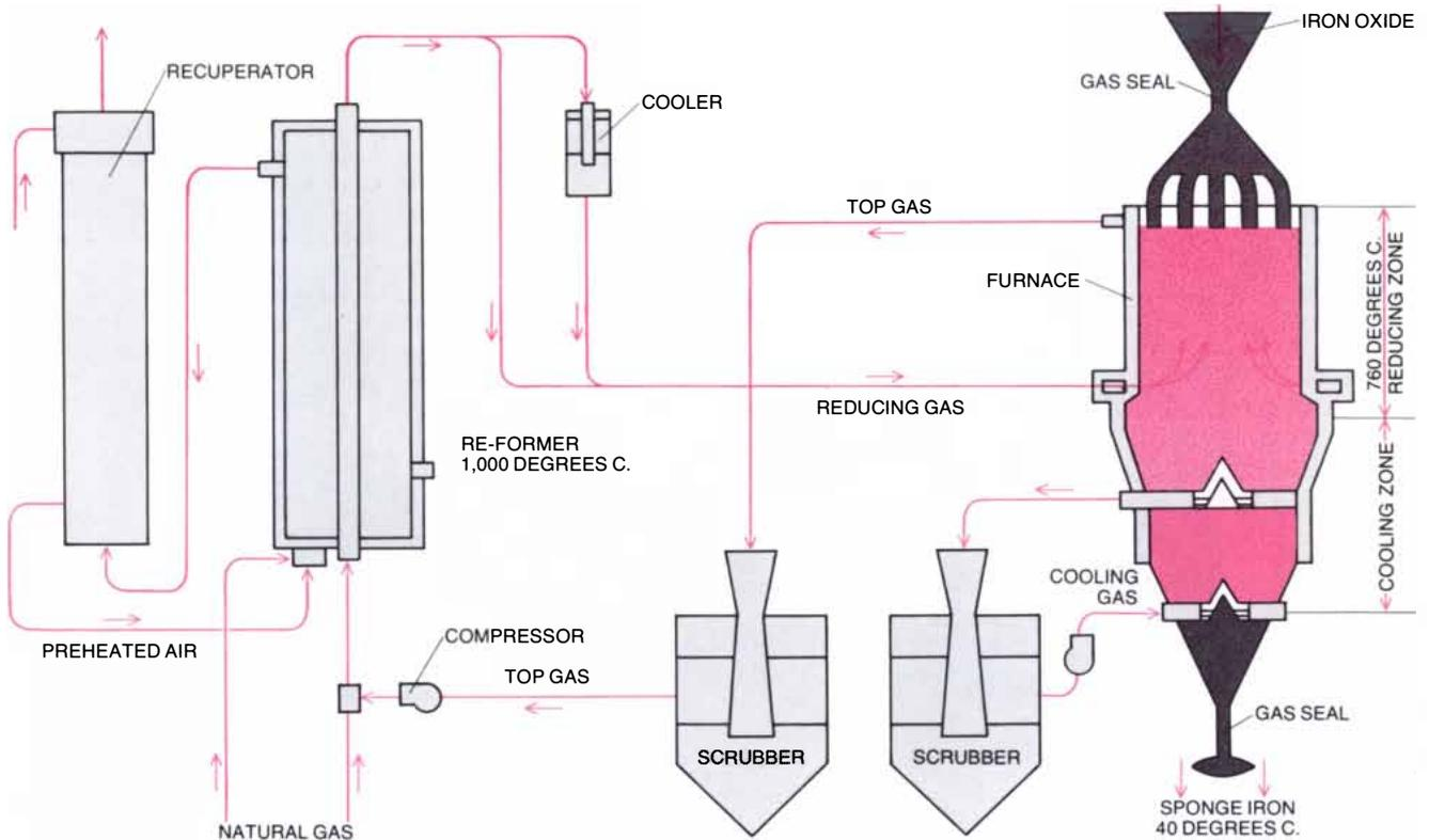
**MIDREX PROCESS** employs re-formed natural gas as the reductant. The process was named by the Midland-Ross Corporation, which developed it. The reducing gas is made in the re-former from a mixture of natural gas and unused gas recovered from the reducing furnace. The furnace is a vertical shaft. A charge of iron pellets and lump
