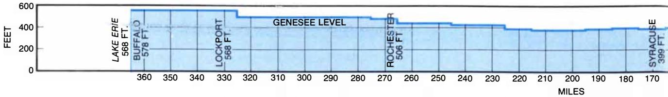
**PROFILE OF THE ERIE CANAL** shows a lift of 568 feet over a distance of 350 miles between the Hudson River (right) and Lake Erie at Buffalo (left). Most of the lift, 425 feet, lay in the 100 miles between the Hudson and Utica, where the major step, 78 feet through
