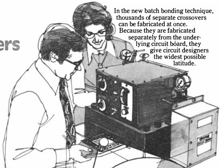
In the new batch bonding technique, thousands of separate crossovers can be fabricated at once. Because they are fabricated separately from the underlying circuit board, they give circuit designers the widest possible latitude.
