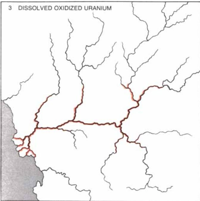
the proliferation of photosynthetic algae increased the concentration of oxygen in the water. Highly oxidized uranium is more soluble than the reduced form, and the uranium was therefore dissolved and carried downstream (3). It remained in solution
