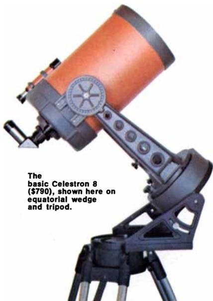
The basic Celestron 8 (\$790), shown here on equatorial wedge and tripod.
