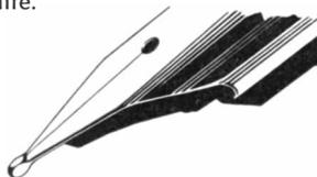
5. Like a fountain pen for writing with flow and character? Remember, the nib is the sensor of the fountain pen. For a smooth feel and even ink flow, it must have some flexibility. The Parker 75 nib is solid 14K gold. Gold has the flexibility and resilience necessary and resists corrosion.
