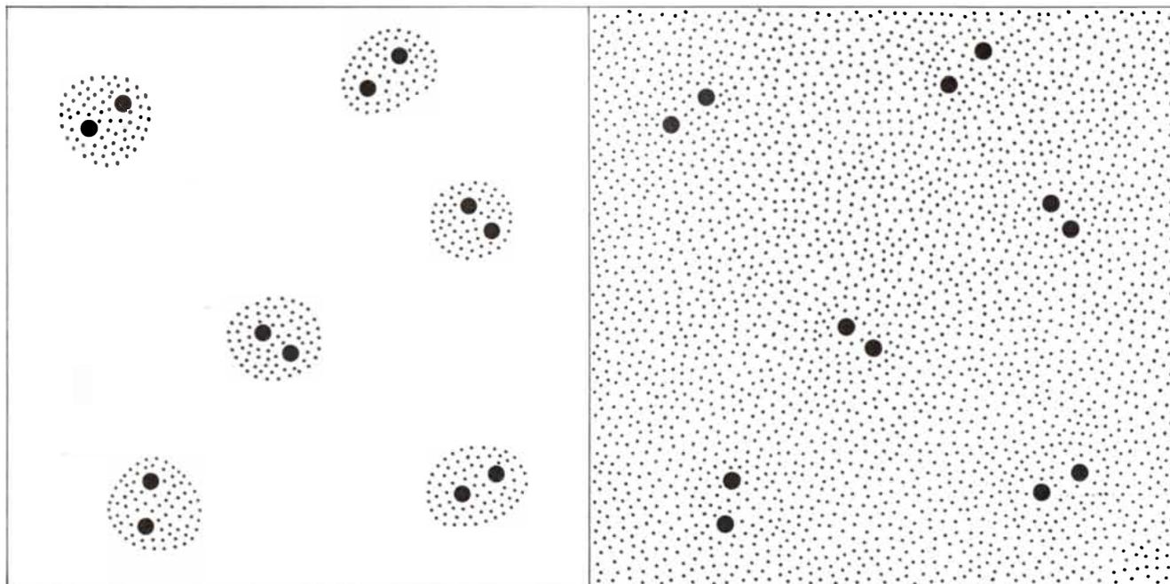
**CONTRAST-MATCHING** is one technique employed to enhance the interference signal in the neutron-scattering data. The interference results from the effective contrast (for thermal neutrons) between the deuterated proteins (*heavy dots*) and the normal proteins (*lighter dots*) in each ribosome subunit. If the subunits are suspended in pure water, however, the neutron beam also detects contrast between the subunit as a whole and the medium, and a spurious com-
