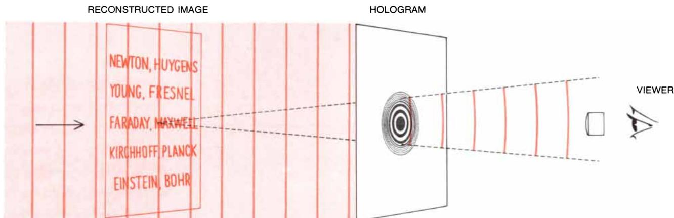
fronts of the reference beam at the photographic plate created a "bull's-eye" pattern resembling a Fresnel-zone diffraction plate. The resulting hologram is an overlay of many such patterns, one for each resolution element of the original object. The diagram at the right shows how the developed holograms were viewed. The diffrac-
