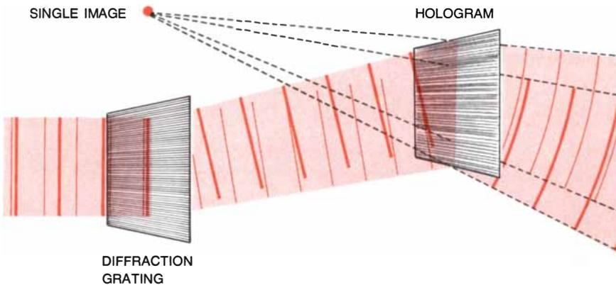
**LATERAL DISPERSION IS CORRECTED** by inserting an actual diffraction grating in the path of the incident light beam. The grating is carefully chosen to have a spacing equal to the average spacing of the fringes of the hologram. Hence it can be used to bend the light oppositely from the way the hologram does, exactly compensating for the lateral dispersion caused by the hologram. As a result images formed at two different wavelengths are focused at same point.
