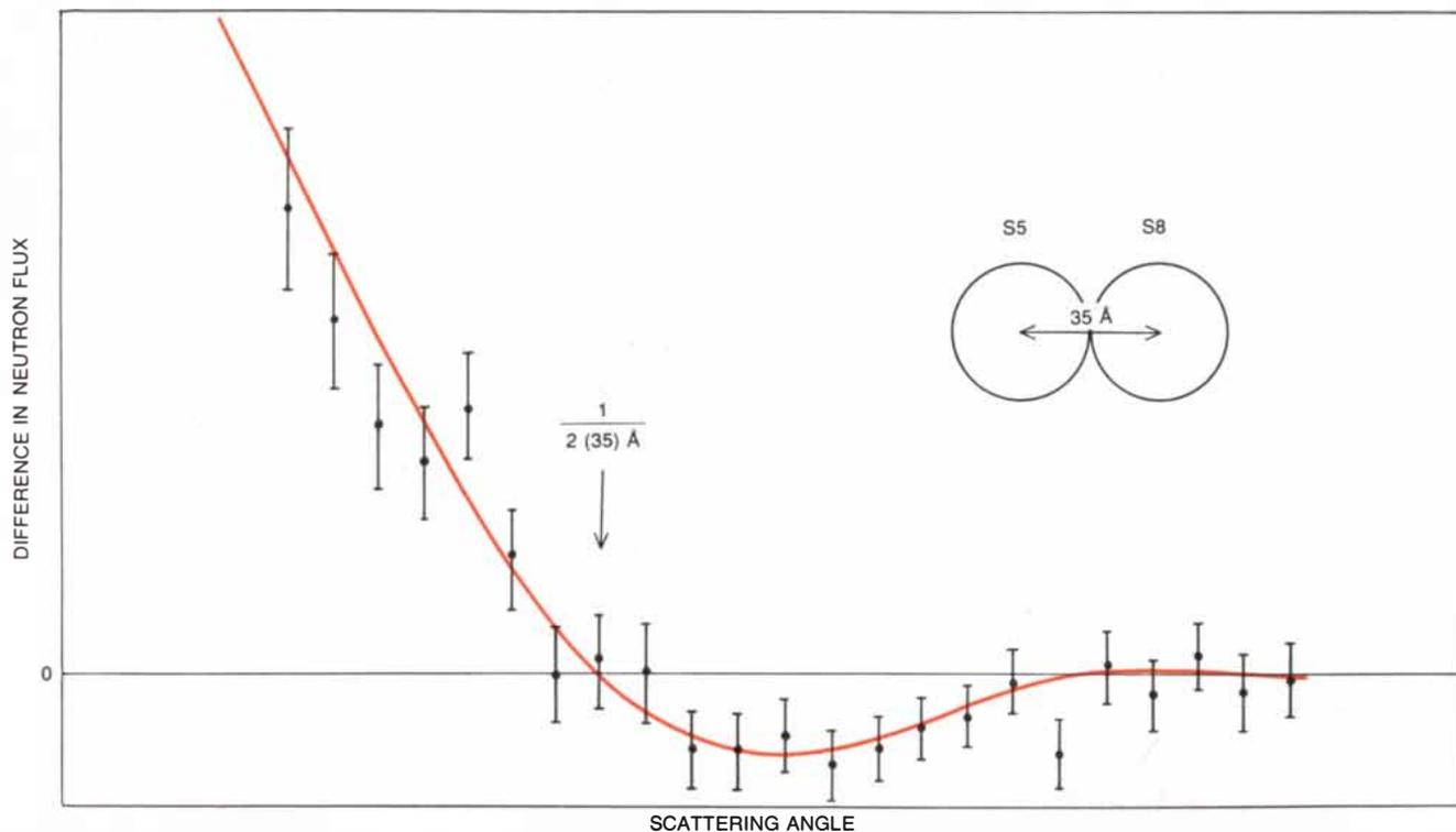
**DISTANCE MEASUREMENT** between two components of the small subunit, the proteins designated S5 and S8, gives a center-to-center separation of 35 angstroms. The measured interference curve is given by the black dots and the vertical bars representing the possible experimental error. The solid curve is a theoretical one calcu-
