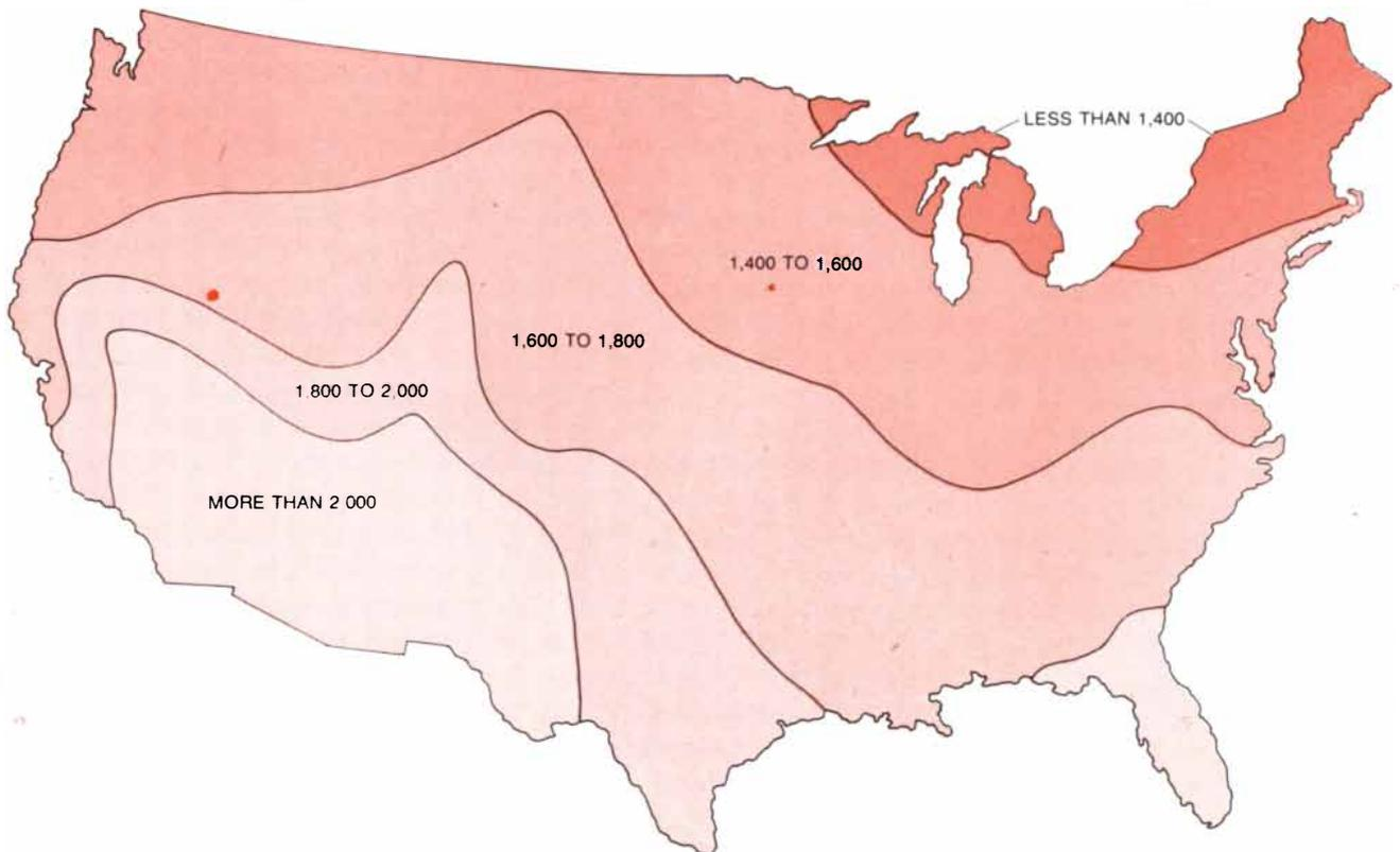
**AMOUNT OF SOLAR RADIATION** received each year in different areas in the U.S. is given in terms of kilowatt-hours per square meter. The amount received in the New England states is about two-thirds the amount received in the southwestern states. In every area,
