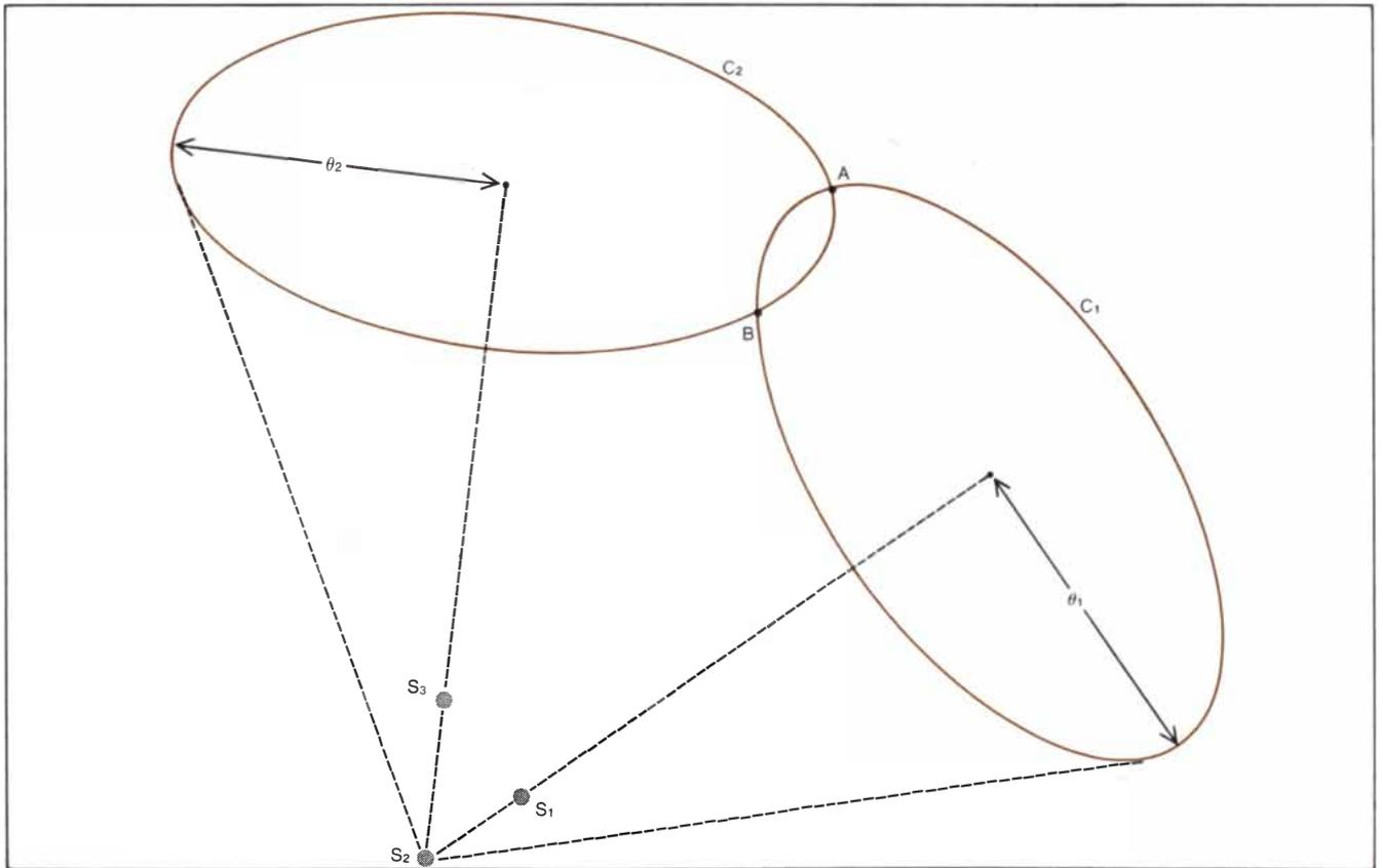
**FURTHER RESTRICTION IN LOCATION** of a source can be accomplished if an event is recorded by three satellites. The difference in arrival times at one pair of satellites, say  $S_1$  and  $S_2$ , yields angle  $\theta_1$ , which determines the size of one circle in space,  $C_1$ , whose center is on a line joining the two satellites. The difference in arrival times at another pair of satellites,  $S_2$  and  $S_3$ , yields angle  $\theta_2$ , which determines
