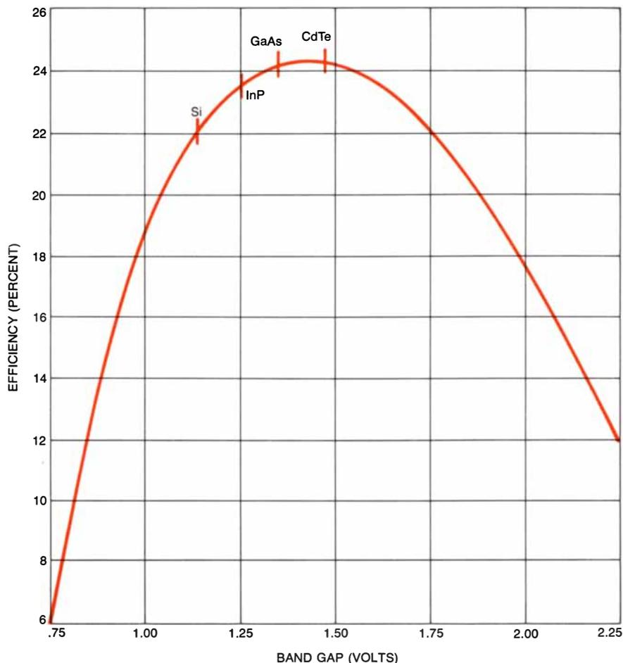
**THEORETICAL MAXIMUM EFFICIENCY** of a photovoltaic cell depends on the band gap of the semiconductor of which it is made. The band gap is given in terms of electron volts. In this diagram the efficiency of four different semiconductors is shown: silicon (Si), indium phosphorus (InP), gallium arsenide (GaAs) and cadmium tellurium (CdTe). Fundamental restraints of physics limit efficiency of even an ideal photovoltaic cell to less than 25 percent.
