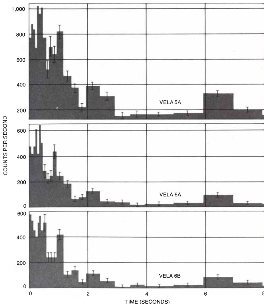
**TRIPLE RECORDING** of a gamma-ray burst was made by three Vela satellites on August 22, 1970. The cesium-iodide gamma-ray detectors begin storing data only if the count rate rises steeply in any given quarter second. The counts are then stored in a sequence of time slots that systematically double in length. It can be seen that the fine structure of the burst, the seventh to be observed, is recorded in the same way by the detectors on all three of the satellites.
