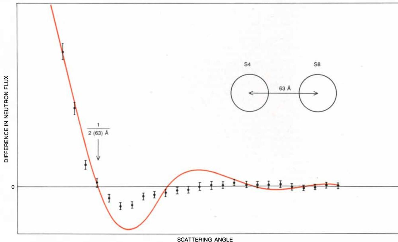
**PROTEINS S4 AND S8** were paired for a second distance measurement. Again the dots and error bars are measured data and the solid curve is based on a theoretical calculation. In this case, however, the theoretical curve is not in good agreement with the data; in particular the measured curve seems to be more strongly damped than the calculated one. The discrepancy probably indicates that one of the pro-
