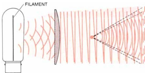
**EXTENDED LIGHT SOURCE** can be thought of as a collection of point sources, each illuminating a point object from a slightly different direction. The bull's-eye patterns are projected in slightly dif-
