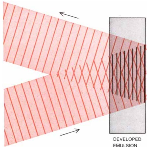
**LIPPMANN PROCESS** for color photography, invented by the French physicist Gabriel Lippmann in 1891, produces interference fringes in a thick photographic emulsion by allowing the incident light to reflect back on itself with the aid of a pool of mercury on the back side of the emulsion (diagram at left). Silver deposits formed at
