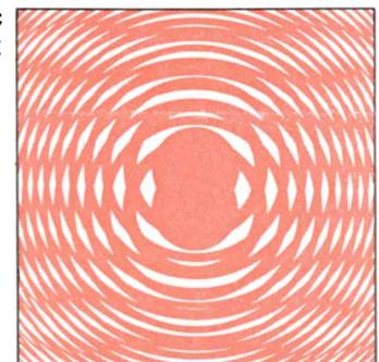
ferent directions and hence are displaced on the hologram. Thus a spatially incoherent, or extended, light source yields a smeared pattern, with finest interference fringes being the ones obliterated first.
