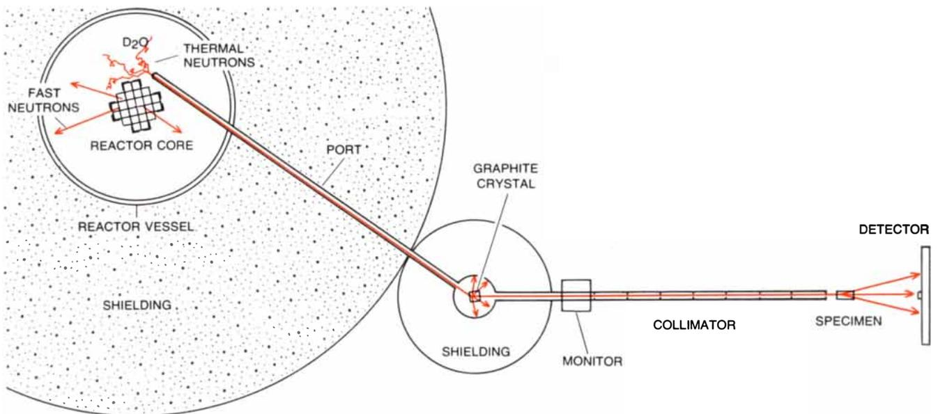
**NEUTRON BEAM** employed in studies of the ribosome is generated by the High Flux Beam Reactor at the Brookhaven National Laboratory. The neutrons are emitted by fissioning nuclei of uranium 235 in the reactor core. They are slowed by multiple collisions with nuclei in the blanket of heavy water that surrounds the core and pass out of the reactor vessel through a port. The distribution of energies among
