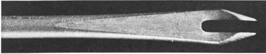
**BIFURCATED NEEDLE** was the principal tool of the vaccination program. The simple instrument was developed by Wyeth Laboratories. The pronged end of the needle is enlarged about 10 diameters in this photograph; the actual length of the needle is about two inches.
