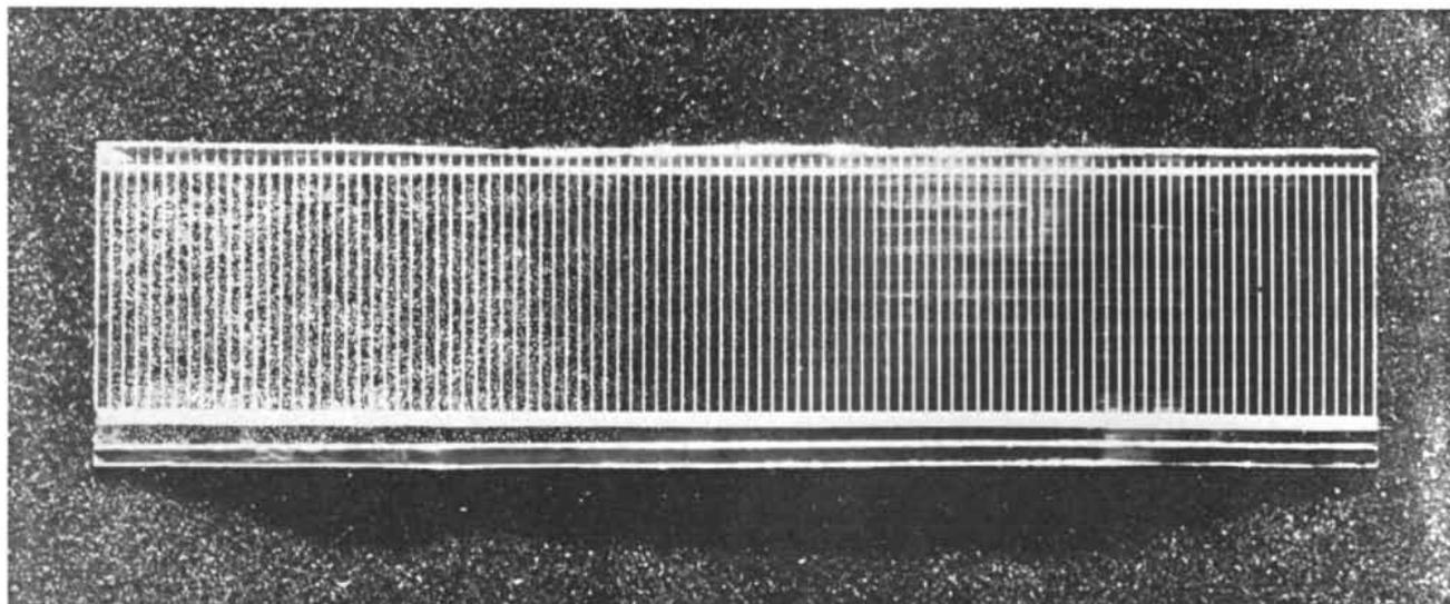
**EXPERIMENTAL SOLAR CELL** made of silicon grown by a new process known as edge-defined film-fed growth (EFG) was made at the Mobil Tyco Solar Energy Corporation in Waltham, Mass. The EFG process is one method that shows promise of lowering the cost of building photovoltaic power stations to a level comparable to the
