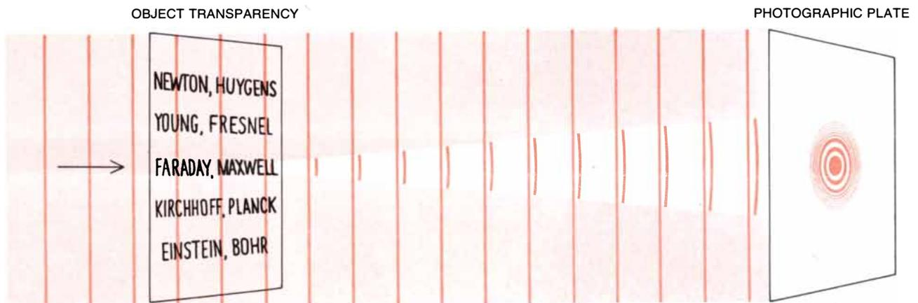
**ORIGINAL HOLOGRAPHIC METHOD**, invented by Dennis Gabor in 1947, employed simple transparencies with opaque lettering as objects and a mercury-arc lamp as a light source. The diagram at the left shows how the holograms were made. Most of the light passed through the transparency and served as the reference beam.
