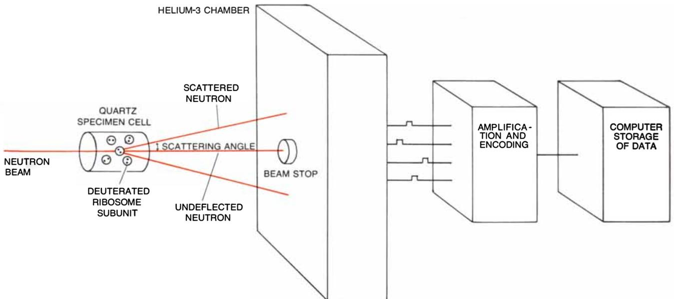
**NEUTRON DETECTOR** records the intensity of the neutron flux at each of more than 8,000 positions on its surface, and thereby measures the angular distribution of the neutrons scattered by the deuterated ribosome subunits. The detector is a flat chamber filled with helium 3, an isotope of helium that emits a proton when it is struck by a neutron. The electric charge of the recoiling proton induces a
