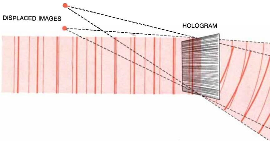
**OFF-AXIS HOLOGRAM**, which was invented by the author and his colleague Juris Upatnieks in 1960, behaves like a parallel-line diffraction grating, bending the light at an angle that is approximately proportional to the wavelength. Images formed at two different wavelengths are laterally displaced, with longer-wavelength image having greater displacement.
