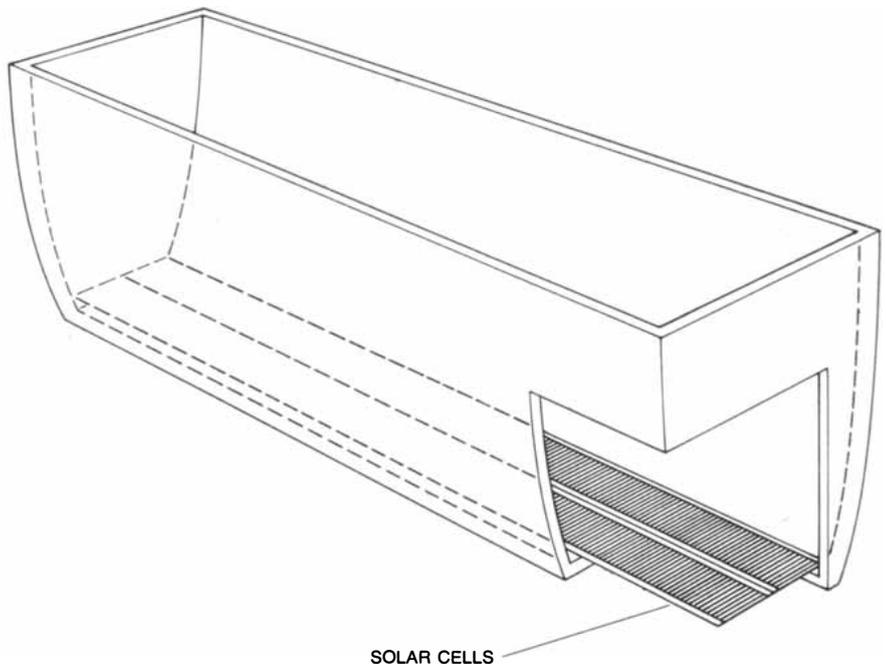
**WINSTON COLLECTOR**, invented by Roland Winston of the University of Chicago, is in the shape of a long trough. It concentrates sunlight on a strip of solar cells and has the advantage that it does not need to be rotated in order to follow sun across sky in course of the day.
