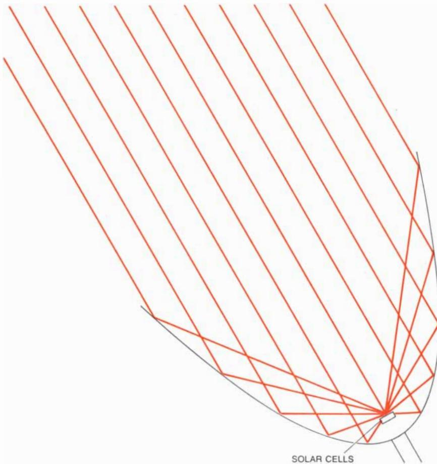
**PARABOLIC REFLECTOR** is one device for concentrating sunlight onto an array of solar cells in order to cut down the number of cells. Such a reflector has the disadvantage that in order for it to work well it must have an automatic driving mechanism to keep it pointed at sun.
