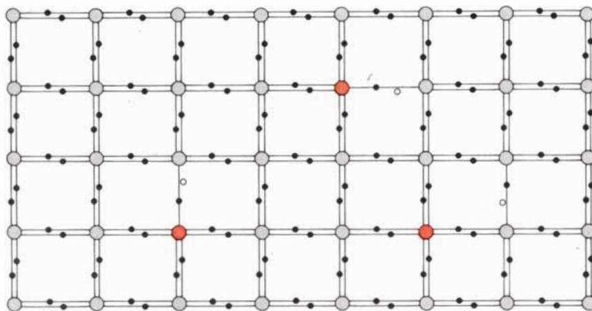
**CRYSTAL OF P-TYPE SILICON** can be created by doping the silicon with trace amounts of boron. Each boron atom (dark color) has only three valence electrons, so that it shares two electrons with three of its silicon neighbors and one electron with the fourth. Hence the *p*-type crystal has same structure as pure silicon, but it contains more holes than conduction electrons.
