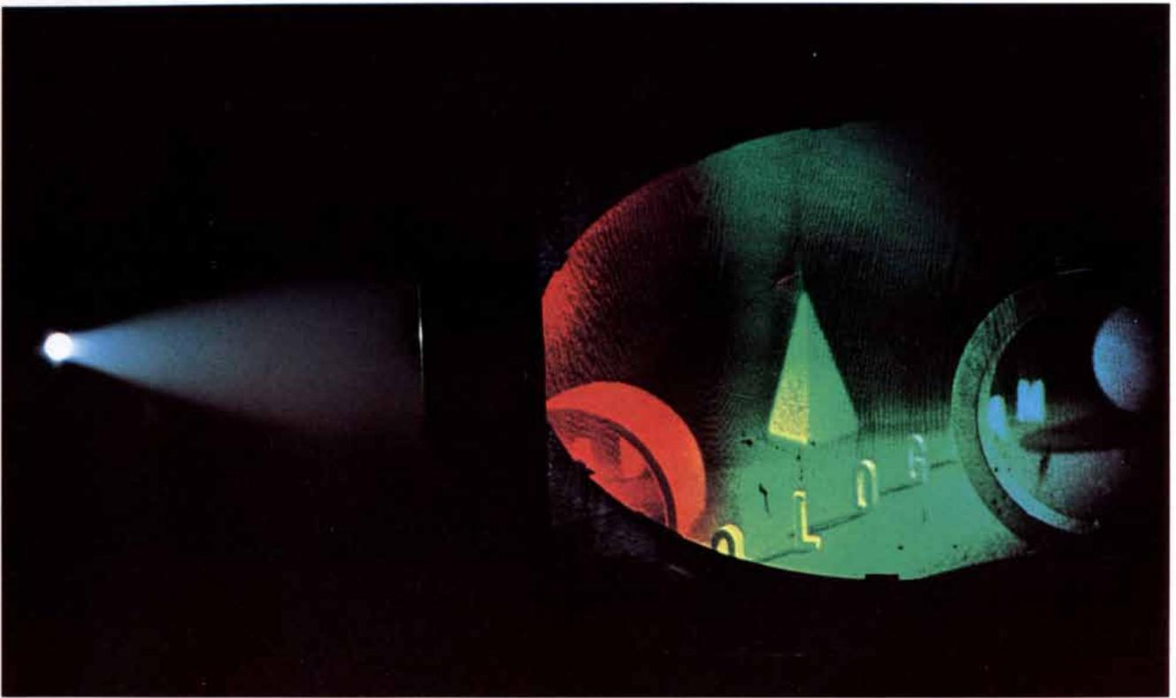
**RAINBOW HOLOGRAM OF SAME SCENE** as the one that appears in the photographs of the conventional hologram on the preceding page was also made in the author's laboratory. When a hologram of this type is viewed in transmitted white light from a distance
