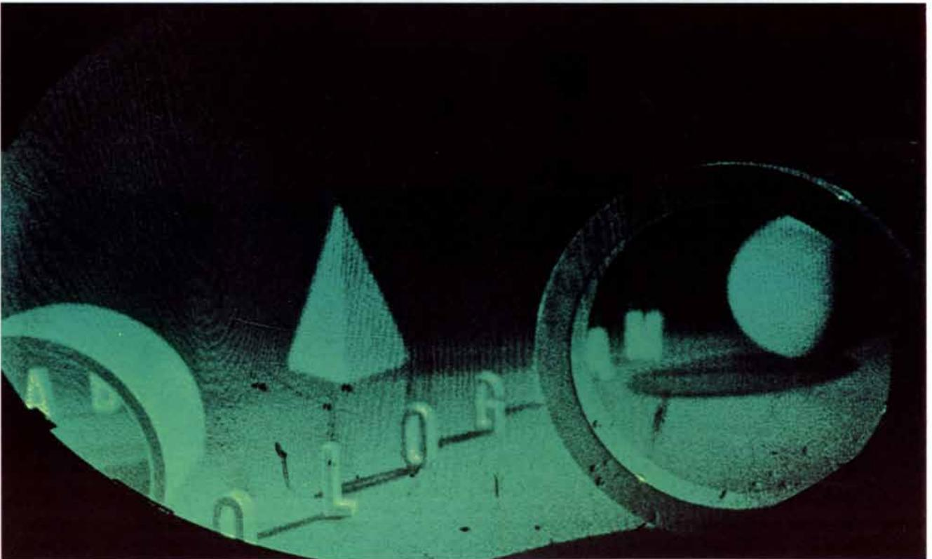
**CLOSE-UP OF THE RAINBOW HOLOGRAM** shown at the top of the page, photographed here with the same tungsten-filament white-light source but now from a distance of about 1½ feet, appears to be uniform in color across the entire image. If one were to
