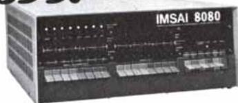
Here is a professional digital computer for home or business use. Complete with front panel, paddle switches, program controlled LED display, 20 amp power supply, card cage, PC Mother Board and documentation. Unassembled, it's \$599. Fully assembled, \$931.
