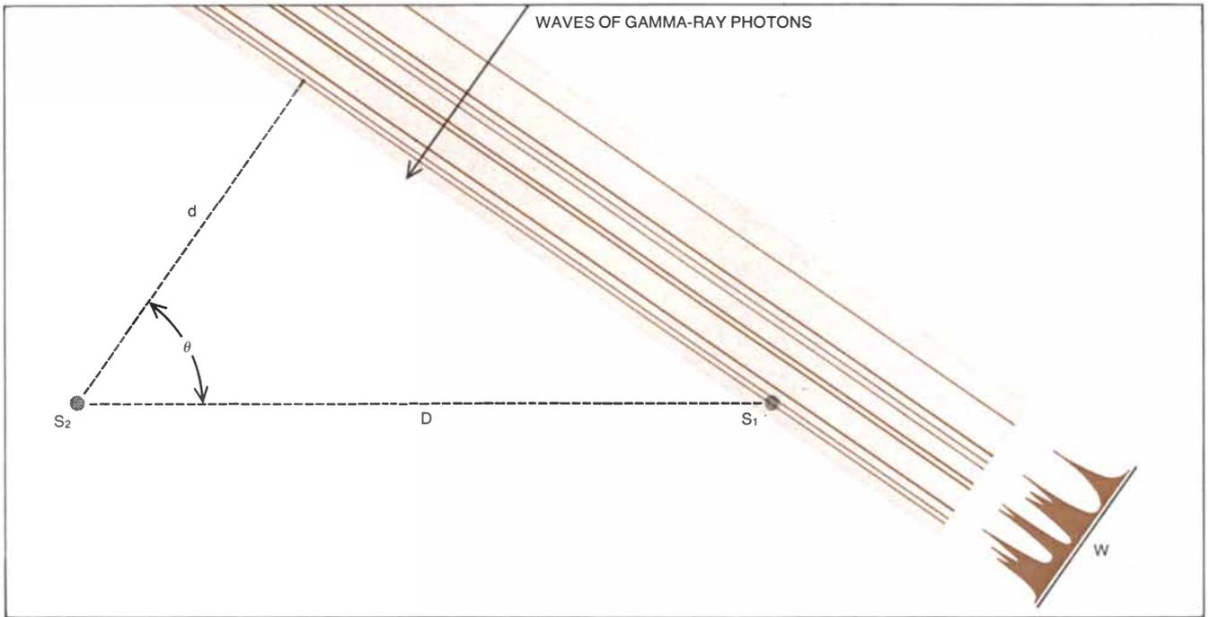
**DIRECTION ANGLE OF GAMMA-RAY EVENT** can be determined if the arrival times of photons from the burst are accurately measured by two satellites whose location in space and separation,  $D$ , are also accurately known. The difference in arrival times yields the distance  $d$ . Knowing  $d$  and  $D$ , one can obtain angle  $\theta$ , the angle the incoming plane wave makes with a line drawn between the two satel-
