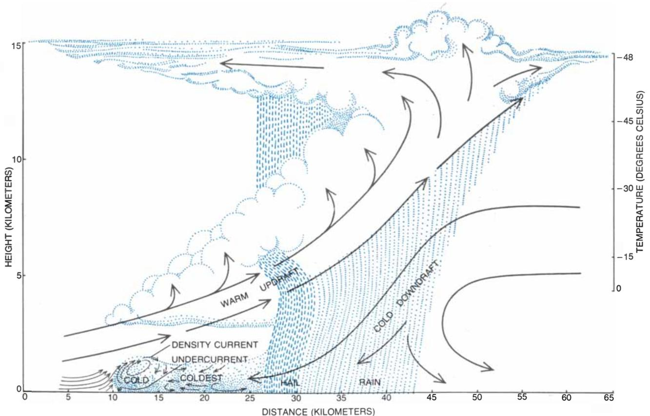
**GENERATIVE MECHANISM** of a dust storm of the squall-line type is depicted schematically. Rain and hail produce a downdraft of cold air that spreads out along the ground and moves forward to form a density current, that is, a body of moving air that is heavier
