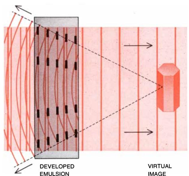
**DENISYUK METHOD** for holography, basically a combination of the Lippmann process and the Gabor holographic process, operates by passing a beam of coherent light through a photographic emulsion, reflecting the light from an object and recording the interfer-
