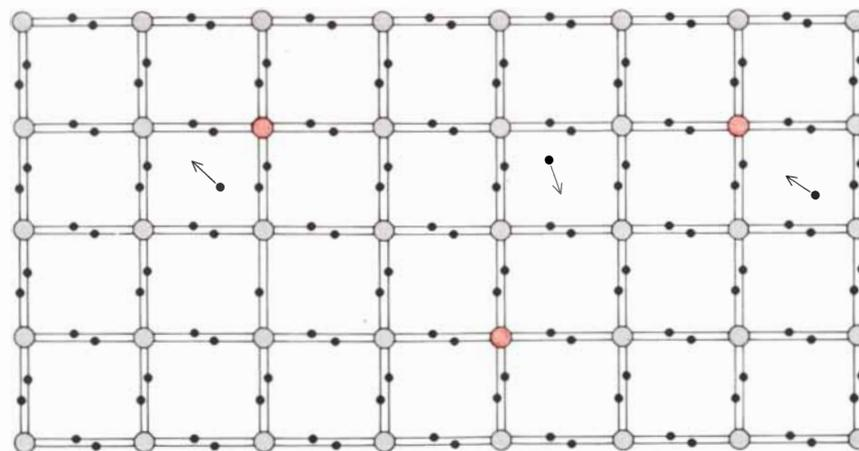
**CRYSTAL OF N-TYPE SILICON** can be created by doping the silicon with trace amounts of phosphorus. Each phosphorus atom (light color) has five valence electrons, so that not all of them are taken up in the crystal lattice. Hence *n*-type crystal has an excess of free electrons.
