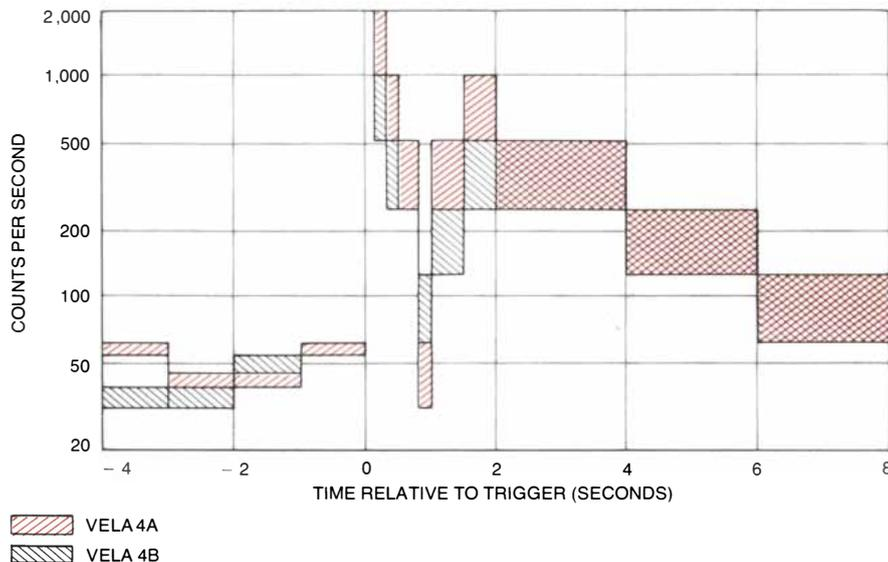
**FIRST GAMMA-RAY BURST** was observed on July 2, 1967, by two Vela satellites, which carried instruments designed to detect radiations of the type that would be produced by a nuclear explosion in space. Responding almost simultaneously, detectors aboard the satellites, traveling in orbit about 250,000 kilometers apart, gave rise to nearly identical responses. Detectors respond to photons in energy range between .2 MeV (million electron volts) and 1.5 MeV.
