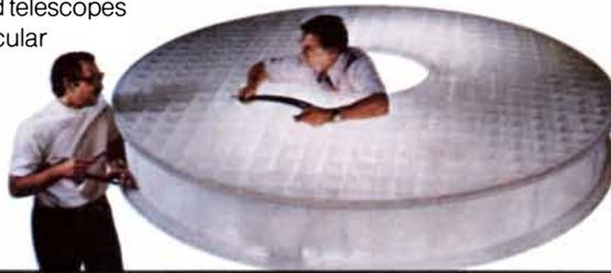
*The telescope's primary mirror will be figured on a precision optical polisher developed by Perkin-Elmer and controlled by a Perkin-Elmer computer.*
