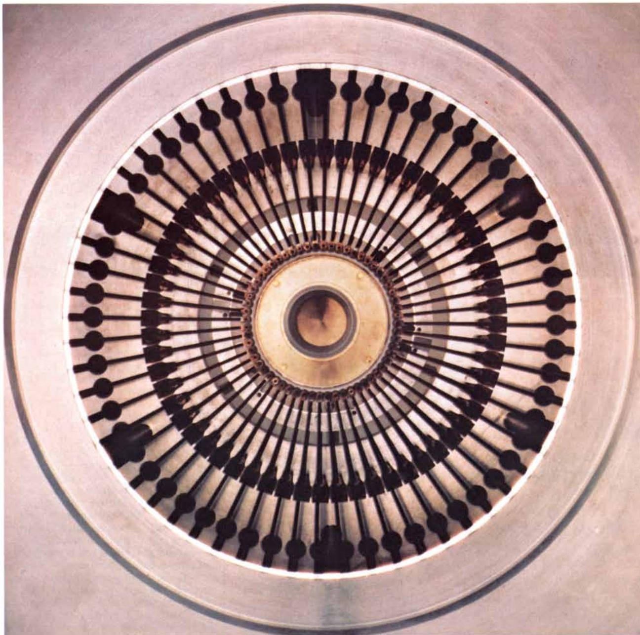
**DETECTOR OF POSITRONS**, or antielectrons, has been employed in the experimental search for events signaling the decay of the vacuum. The portion of the detector visible here consists of 60 small coils, each of which generates a toroidal magnetic field. Positrons are directed by the fields into the central well, where they encounter electrons and are thereby annihilated. The resulting gamma rays, or high-
