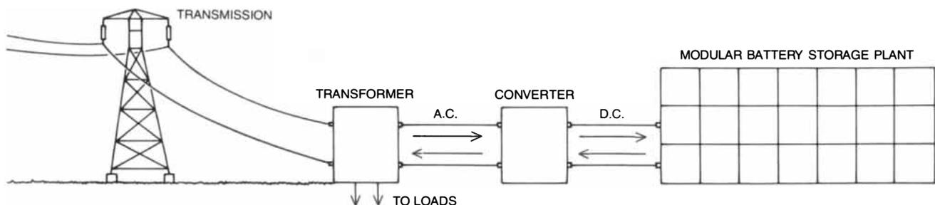
**ENERGY STORAGE IN ELECTRIC BATTERIES** would have many new advantages if the advanced battery systems that are now under development prove to be successful. Unlike pumped-water and compressed-air storage systems, battery storage plants could be put almost anywhere. Since they could be assembled from mass-produced
