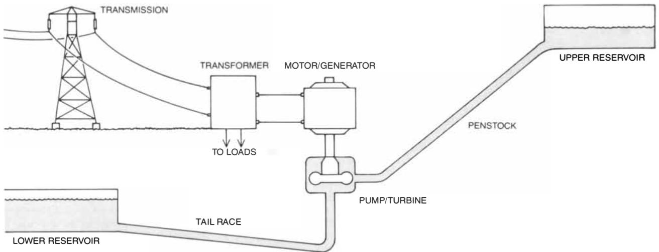
**PUMPED-HYDROELECTRIC ENERGY STORAGE** is the only large-scale electric-energy storage system whose economic feasibility has so far been demonstrated in the U.S. Surplus base-load generating capacity is used to pump water from a lower reservoir to an upper one in periods of low demand. About 35 such systems with a
