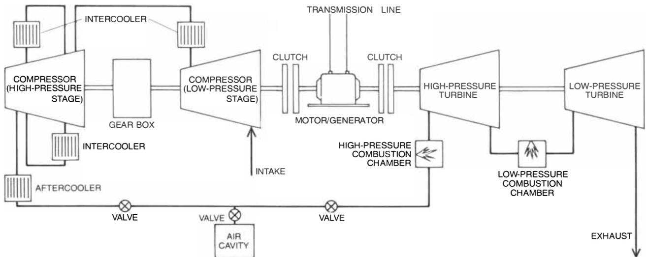
**COMPRESSED-AIR ENERGY-STORAGE PLANT**, the first of its kind, is now operating at Huntorf, near Bremen in West Germany. In periods of low demand (typically over an eight-hour night period) air is compressed and stored at a pressure of about 70 atmospheres in two caverns leached out of a salt dome that have a combined capacity
